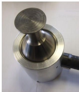
20 kHz, diam 40 mm, Thrust 140 g at 100 W
